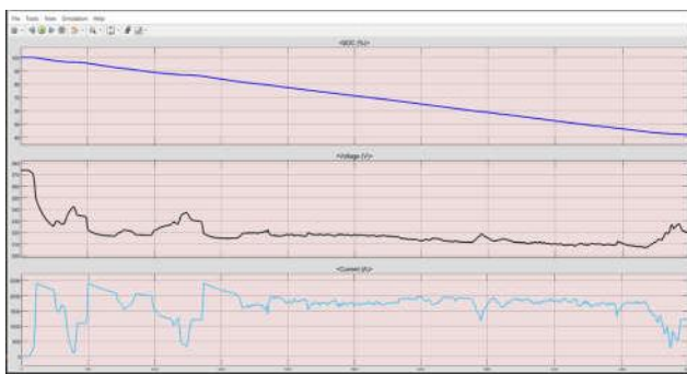
The graph of current, voltage and the SOC (state of charge) in the system, and their comparison.
