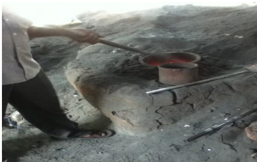
MOLTEN STAGE OF ALUMINIUM
