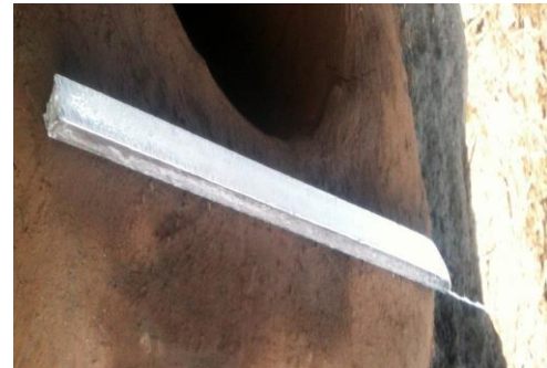
RECTANGULAR ROD AFTER CASTING
