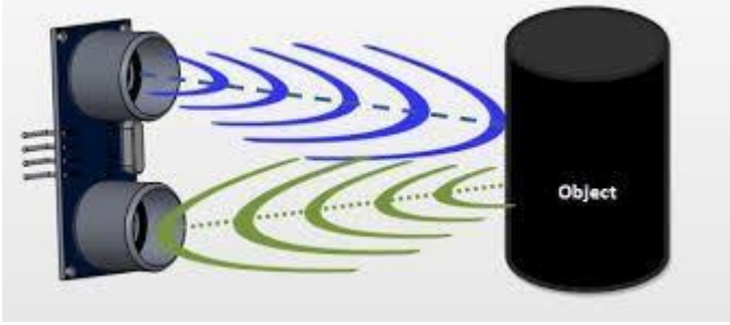
Figure 2: Working of ultrasonic sensor
