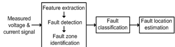
Fig. 6 Block diagram representation of three main stages of a digital distance relaying scheme for the protection of FACTS compensated transmission lines
