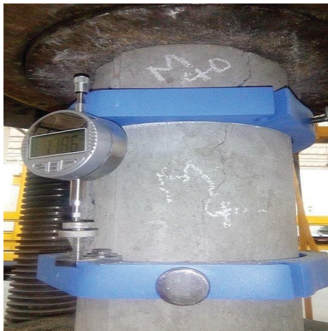
Fig. 2 Test setup for Elastic Modulus.
