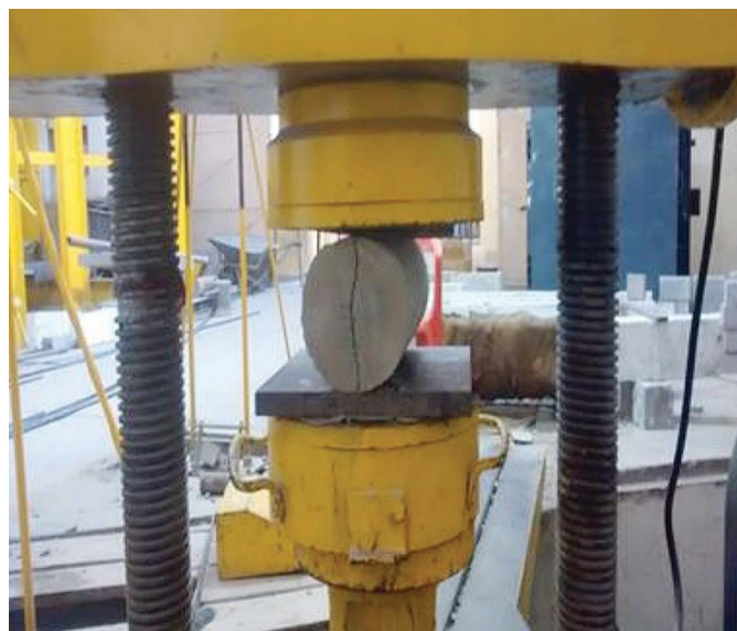
Fig. 4 Test Setup for Split Tensile test.
