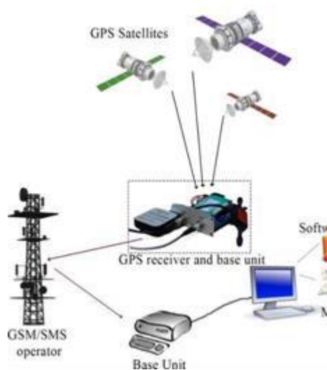
Fig 2: Block diagram of GPS tracking system
