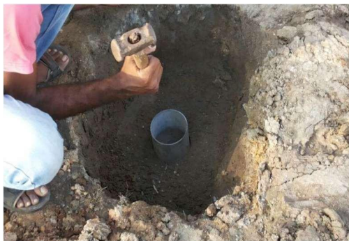
Figure 6. Typical open pits manually excavated using pick-axes and shovels
