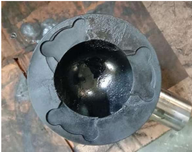
Figure 2.3 Modified Grooved Piston After Combustion
