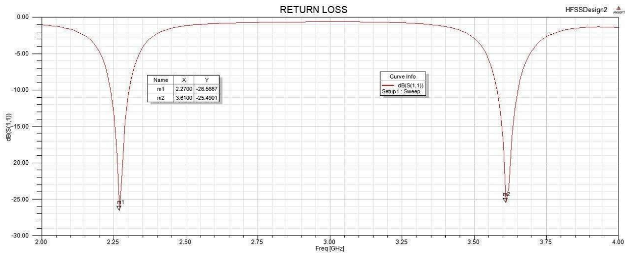
Fig. Return Losses for 2x2 Microstrip Patch Array Antenna
