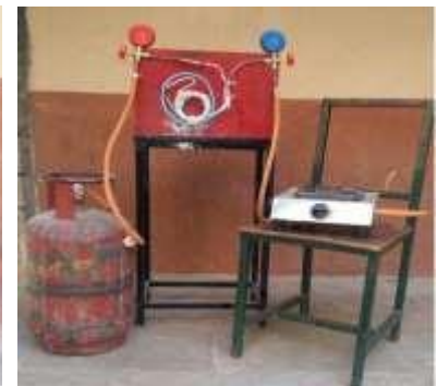
Fig-1: Schematic diagram of simple VCRs Fig-2: Actual Setup of LPG Refrigerator Fig-3: Actual Setup of LPG Refrigerator
