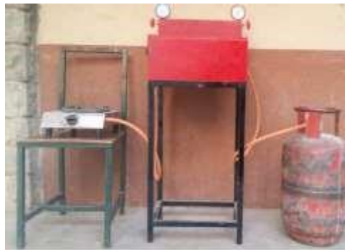
Fig-1: Schematic diagram of simple VCRs Fig-2: Actual Setup of LPG Refrigerator Fig-3: Actual Setup of LPG Refrigerator
