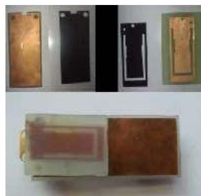
Figure 7. Fabricated designed PIFA before and after assembly.
