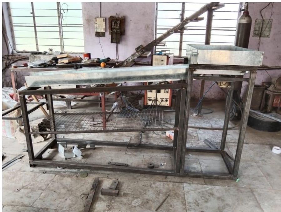
Figure 2. Actual representation of sweet lemon sorting machine
