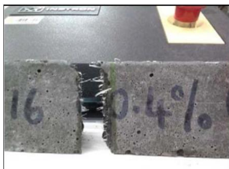
Figure 11: Cross section of samples with fiber after test
