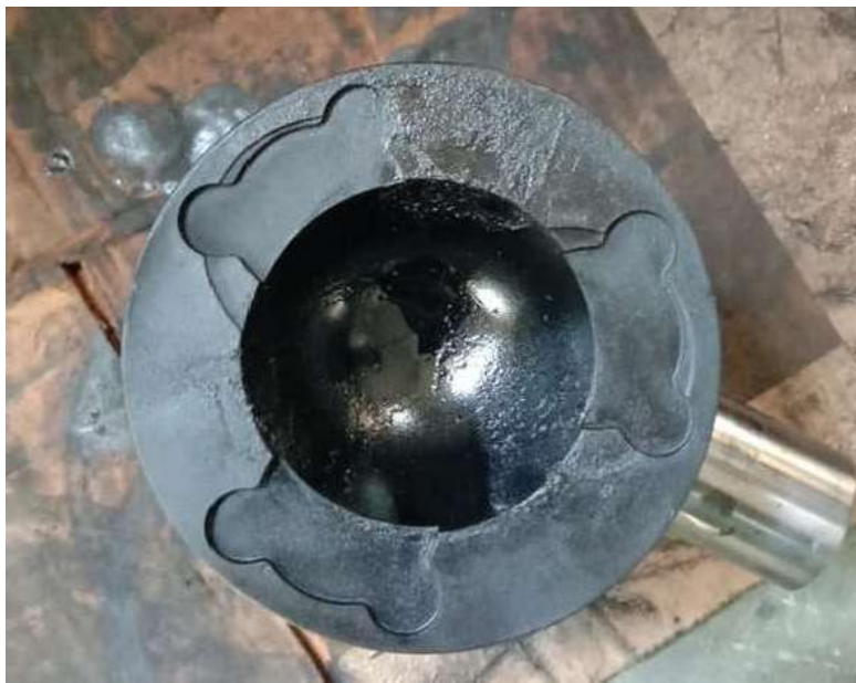
Figure 2.3 Modified Grooved Piston After Combustion
