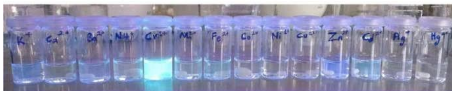
Fig.15. Fluorescence of various cations showing visible sensor strength for \text{Cr}^{3+} and the weakness of interference from other cations.
