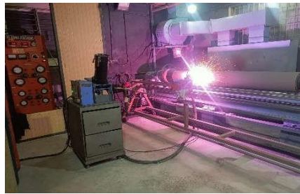
Fig. 8. PLASMA SPRAY TECHNIQUE
