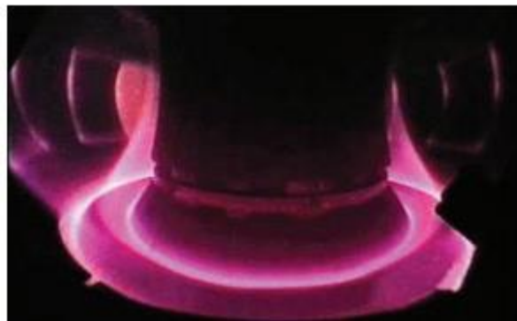
Figure2: Examples of high temperature plasma: the fusion plasma in the tokamak ASDEX (T = 10keV)
