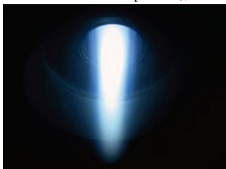
Figure3: Arc discharge of Ar with H 2 plasma (Thermal plasma).
