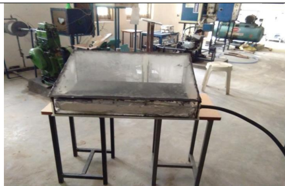
Figure.5. Fabricated Solar Still With Acrylic Material
