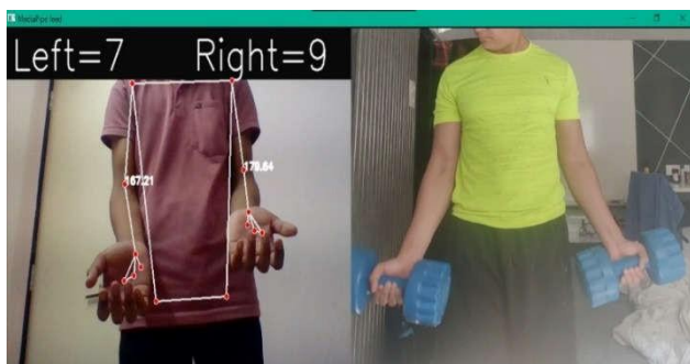
Image – 2 The interface of GYM-AI, user can compare their form to the form of reference video and the GYM-AI program will trigger buzzer when the rep is done incorrectly. This image corrects the form of double bicep curl exercise
