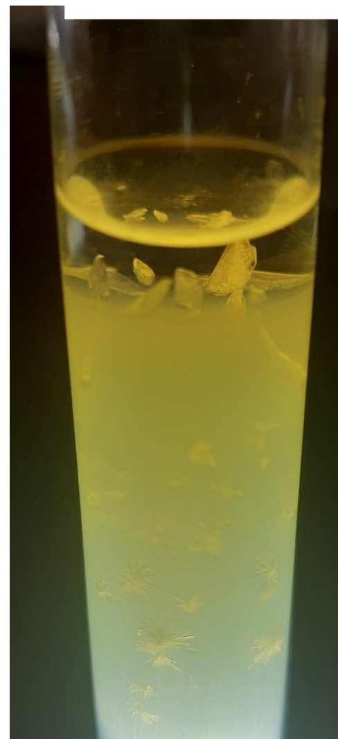
Figure 2. Prismatic platy shaped transparent crystals at the interstitial and spherulites inside the gel.
